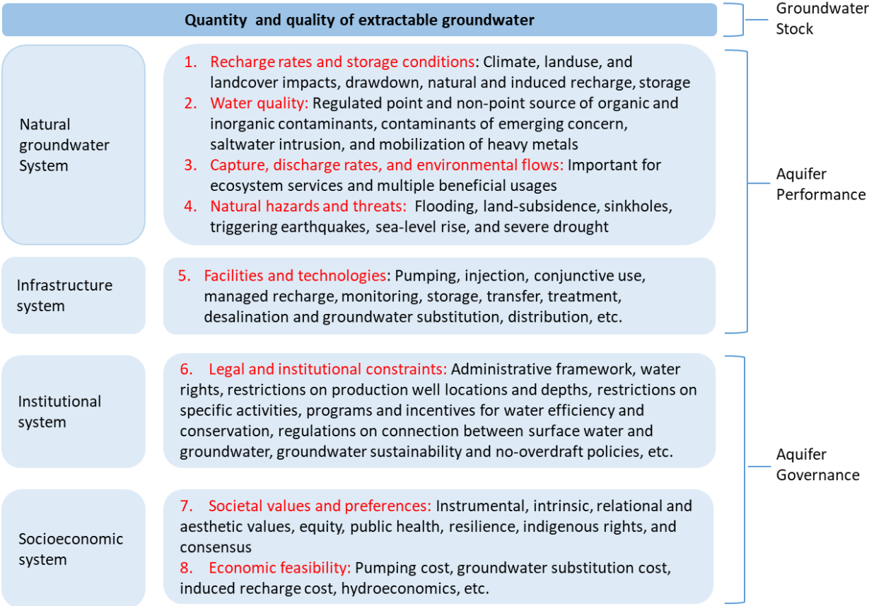
Fig. 3. Factors to consider for groundwater sustainability evaluation modified from (Elshall et al., 2020a)
